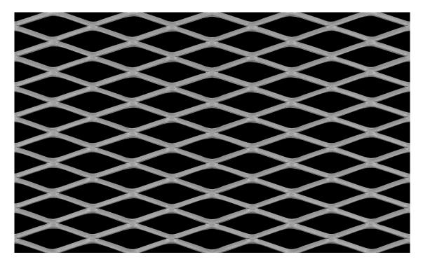
LW Aperture:24.38mmStrand Width:2.39mmSW Aperture:7.11mmThickness:1.14mmWeight:3.64 kg / m2Open Area:60%
